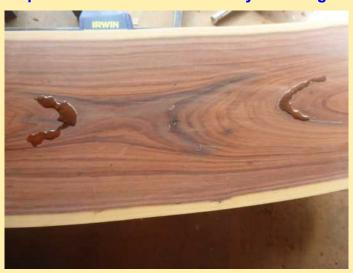
The small cracks were filled using ultra clear E-poxy glue. The larger areas were filled with the same glue, but with a small amount of wood dust mixed in. This was allowed to set overnight.
