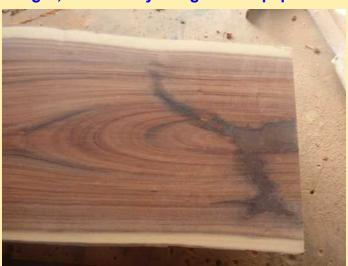
The final sanding was done in the direction of the wood grain for a better finish.
