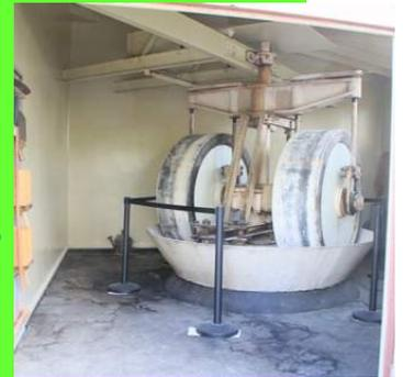
Essentially, the mill consists of two large iron, or steel, wheels held just above an iron, or steel, dish and, as the mill rotates about its vertical shaft that also rotates the large wheels, the powder is mixed and ground. The powder consists of charcoal, sulphur and saltpeter (potassium nitrate).
