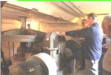
Needless to say, igniting the gun powder would be disastrous, so extreme precautions were needed to reduce the risk of explosion. The electric drive for the mill was installed below the concrete floor and the room was lit by lights installed outside the building which shone through the windows. As well, the powder was wetted during processing.
