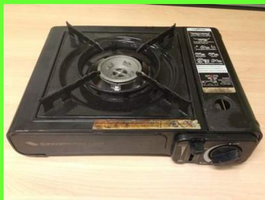
These products are often used when picnicking, camping and caravanning. Recent testing by certifying bodies found the products’ shut-off and safety valves failed to operate once heat was dispersed over the butane gas cylinder. This means they could overheat and possibly explode, causing serious injury. The tests concluded that the products did not meet the safety requirements under the Australian Standards and they have since been removed from sale in NSW.
